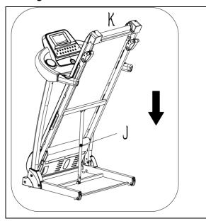
Support place K with a hand, press the frame slightly, then kick the place J, and the base frame will fall down automatically.
