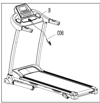
Before running, please insert the Safety Key (C06) into the magnetic area of the Console (B) and fasten the safety key clip (C06) with your clothes.
