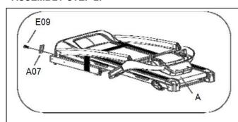
Remove the bolt M8x15 (E09) and Safety block (A07) with Allen wrench (B08)
