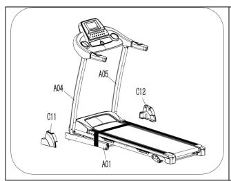
Push the Left & Right upright tube covers (C11, C12) onto the base frame (A01) and Left & Right upright tube (A04, A05).
