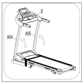
Lift up the console (B) and left & right upright tube (A04, A05) towards the arrow direction.
