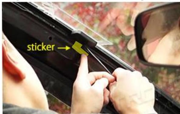
3. Attach the antenna to the windscreen once the copper grounding lug is secure. (Please try to keep the antenna away from the metal ground of the car, at a distance of 60mm at least, and you should place the antenna upward).
