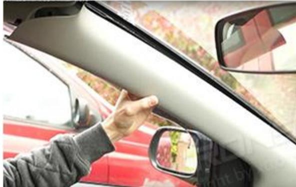
2. Scratch away some paint from the A Pillar to attach the copper grounding lug. (Please tear out the sticker from the grounding lug surface and ensure the grounding lug has good conduction with the car's ground).
