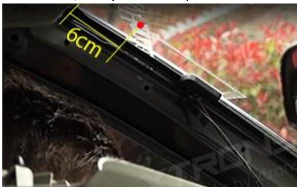
4. Run the cable to the rear of DAB stereo and connect to test. Refit the A Pillar once completed.
