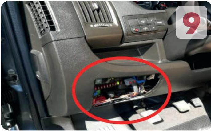
Open the fuse box in the dashboard underneath the steering wheel
