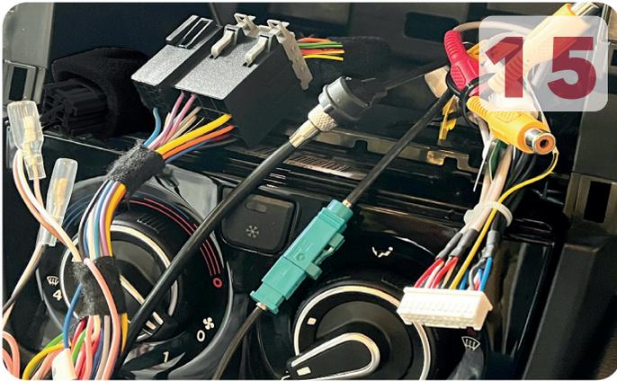
Connect all cables in the dashboard including FM & DAB with the included cables.
