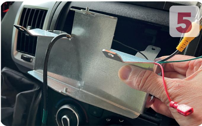
Slide the installation bracket in the dashboard with the bottom side towards you
